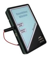
It is simply fastened with a special removable glue strip at the desired place for measurements. The electronic safety device registers any manipulation of the data logger. If readings show a humidity of more than 60 % over a longer period of time, these are the conditions to critical forming fungus. Fungus not only destroys walls, wallpaper, floors and interior fixtures, but they also lead to various illnesses such as allergies and infections.
