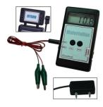
The Materialfox is an efficient and multitalented instrument for recording the humidity situation of a variety of materials. Measuring is done through the measuring peak sensor or with two terminals that are fastened on two specimens. The data logger displays and records either the current resistivity or the relativ humidity value (humidity equivalent) of the material analyzed.
