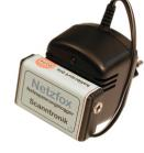
The Netzfox is an electronic data logger that registers the voltage of the 230-V power system continuously simply by plugging the device into the wall socket. The PC software allows a detailed graphic analysis of the voltage
