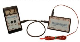
and the reading of the measuring results. Parameters, such as the measuring interval, the date, the calendar or the hysteresis, can be set with the help of the PC software which is available separately.
