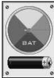
Figure 5: The Rissfox Mini's battery indicator
