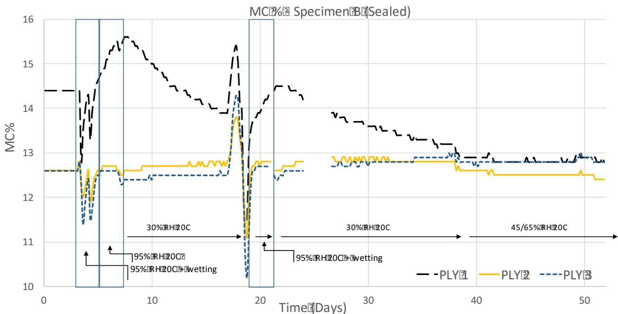
Figure 3: Moisture curves of specimen B – sealed over the duration of 52 days
