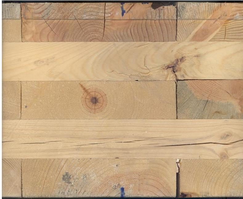
Figure 7: Checking, gap widening, material defect, and delamination in edge condition
